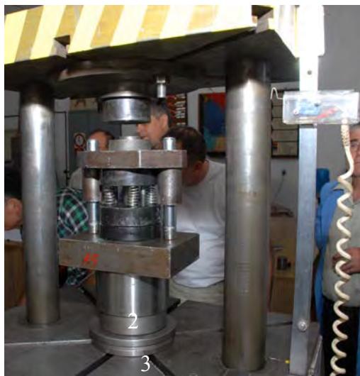
Fig. 2. The experimental lobe die: 1-hydraulic press, 2-lobe die, 3-resistive force transducer
