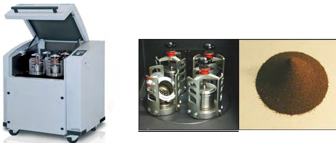
Fig. 3. Retsch machine and steel vials for preparing mixed powder of Cu7Ag 0.05Nb for compressed rods
